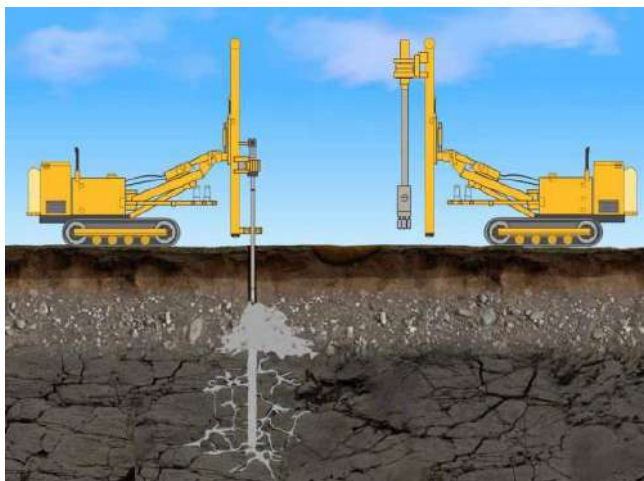
Fig. 3. High-pressure soil injection.
