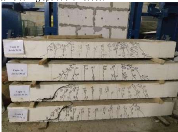
Fig. 5. Experienced beams after testing.
