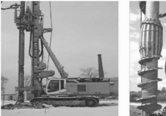
Fig. 4. Baue drilling rig for pile compaction and its working body.
