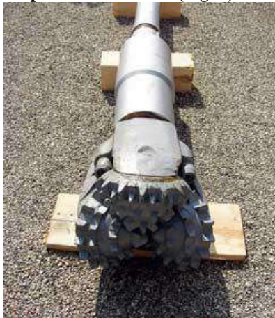
Fig. 1. Hollow drill rod for delivering mud to the well.
