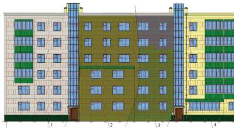
Fig. 2. Conditional scheme of insulation of the facade of the building (from scaffolding): 1 – cleaning of the facade from dust and dirt, remnants of the existing insulation, surface repair; 2 – priming the surface of the facade, gluing insulation plates, fastening with dowels; 3 – application of the 1st layer of plaster, gluing of the reinforcing mesh, application of the 2nd layer of plaster; 4 – priming, application of decorative finish
