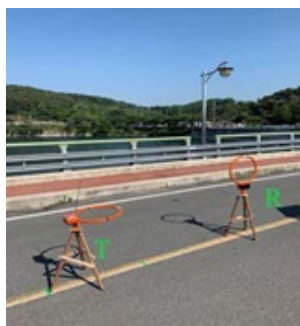
Fig. 2. Ground Penetrating Radar SDI K-5 on the dam at Nonsan. T is the radio wave transmitter; R is the receiver.
